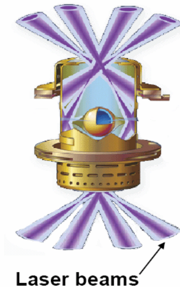
NIF glass laser Ignition hohlraum
