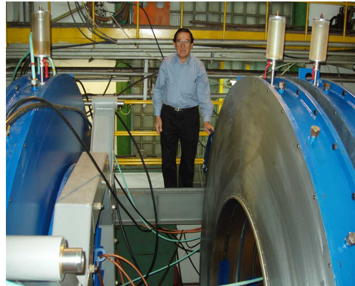
Test stand for Voltage adder testing of five 1.0 MA LTD cavities (High Current Electronics Institute – Tomsk, Russia)
