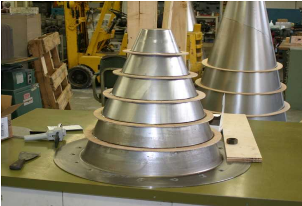
Stiffening rings mounted to PoP- RTL cone
