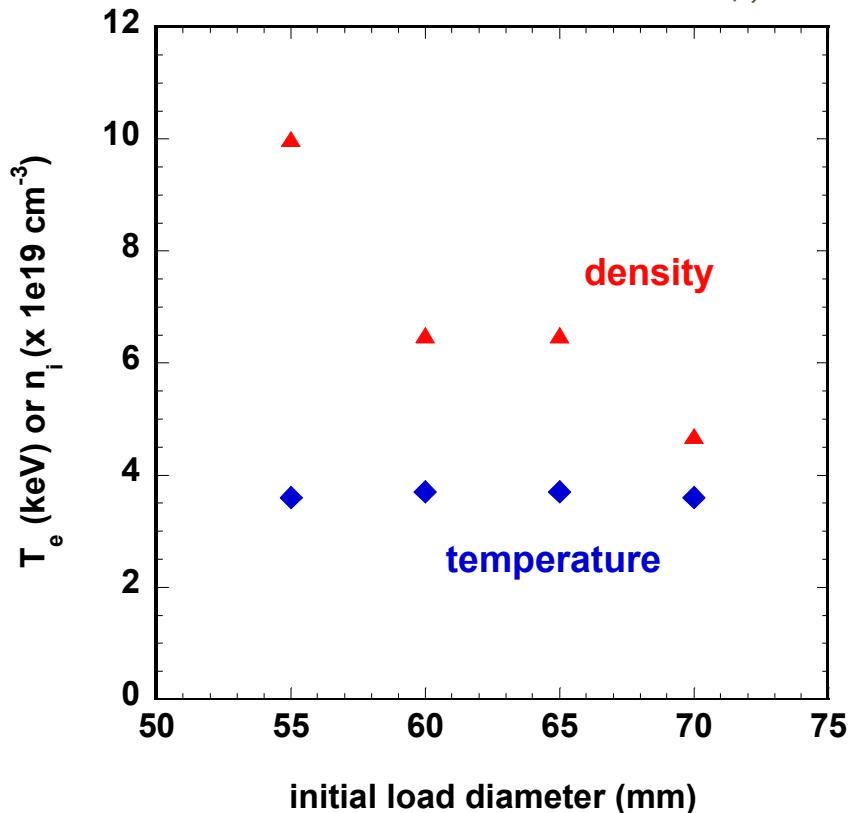
There was not a significant change in  $T_e$  over the range of wire numbers that could be fielded, but  $n_i$  increased with smaller wire number
