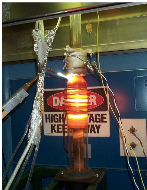
Figure 16. CVD reactor in operation during initial deposition of NbC into TaC foam.
