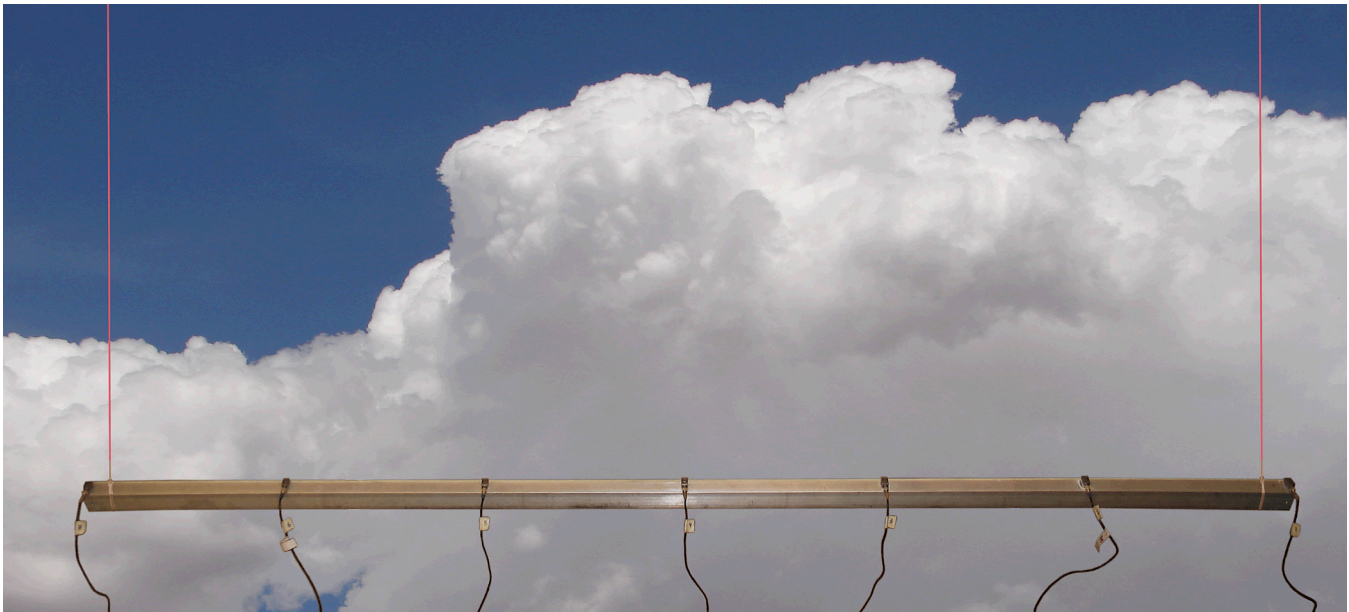
Figure 3: Photo of Lightly Damped Aluminum Beam with Variable Length Elastic Supports
