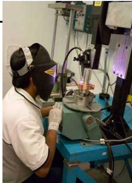
Putting a Closure Weld on a Thermal Battery
