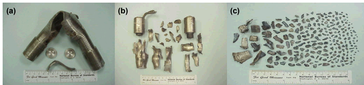
Figure 1. Examples of cookoff responses: (a) mild pressure burst [PBXN-109, 3°C/hr], (b) moderate violence [PBX9501, 195°C hold] (c) high violence, detonation-like response [LX-10 at low pressing density, 3°C/hr].
