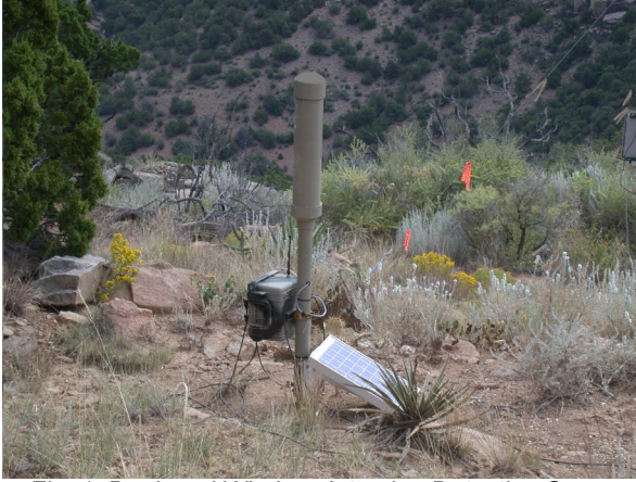
Fig. 1. Deployed Wireless Intrusion Detection Sensor B. Sensor Node Power Supply Model
