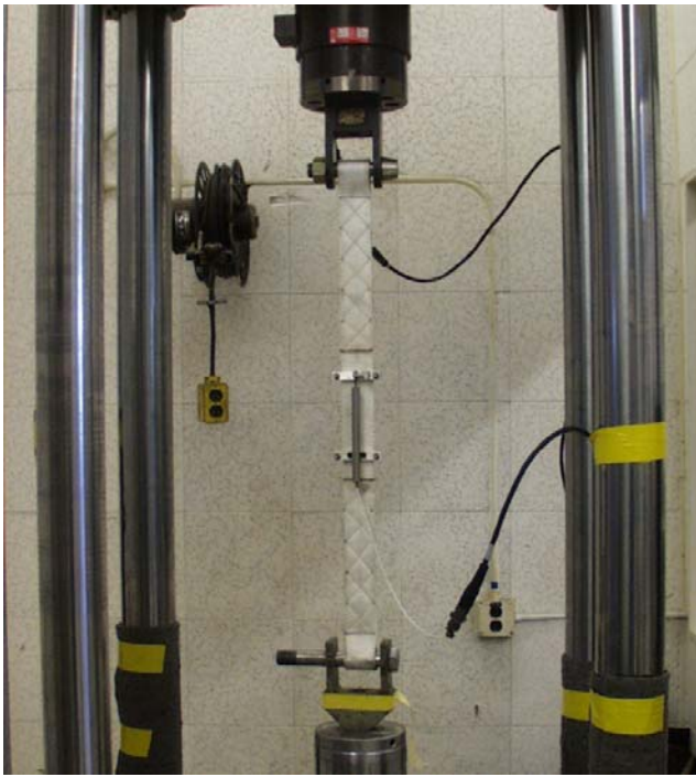
Figure 2. Load elongation measurement setup
