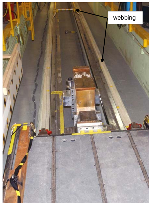
Figure 6. Left: impact sled. Right: configuration for calibration shot, showing nylon loop crossing track, and impact sled in position with column extending beneath the test-item platform
