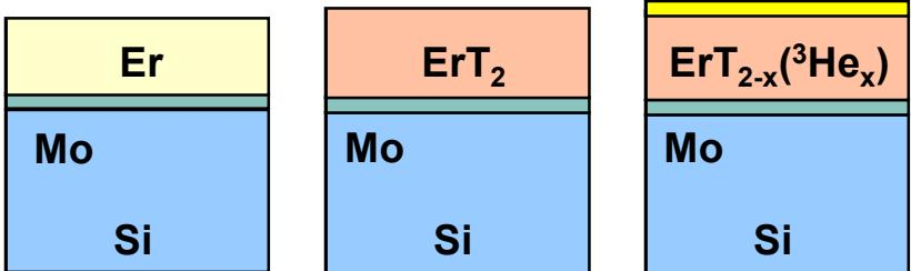
Oxide forms during hydriding and upon air exposure.
