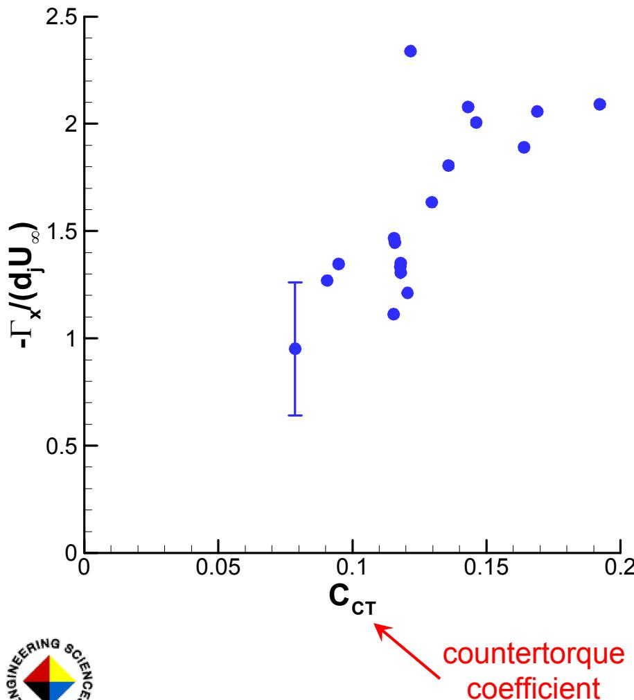
This suggests that jet/fin interaction arises from an induced angle of attack on the fins,  $\alpha_{fin}$ .
