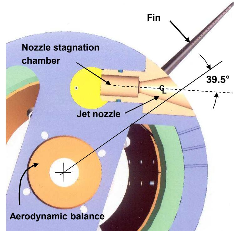
Cross-section through plane of spin rockets
