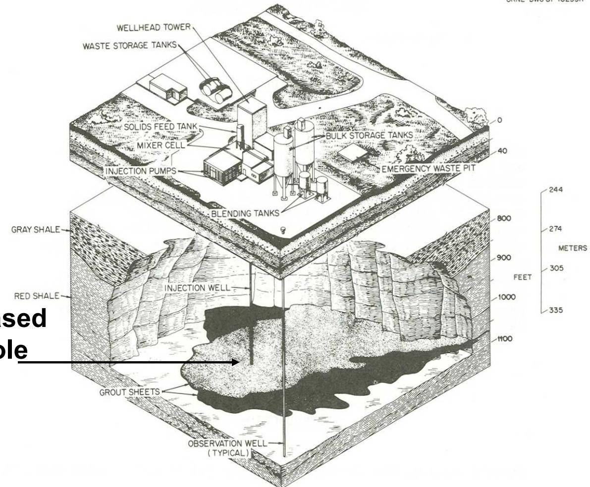
**Fluid Portland cement based grout is injected down hole at sufficient pressure to hydrofrac the formation.**
