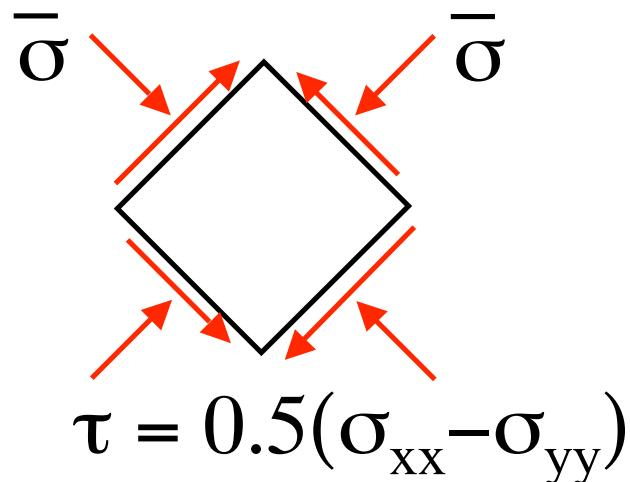
By a simple tensor transformation (45° rotation), the stress state can be expressed as a mean stress (mechanical pressure) and a shear stress
