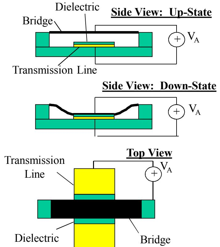
**MEMS switches pair the performance of electromechanical switches with low cost and size of solid state switches.**
