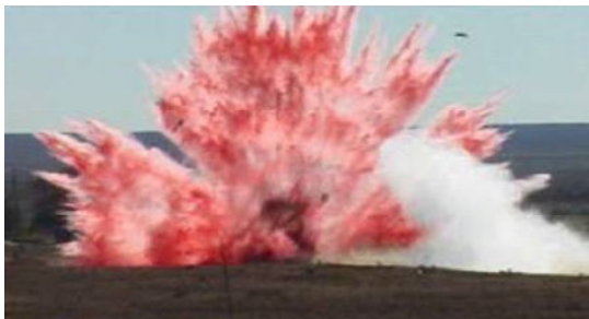
Figure 1. Dispersed water (dyed red) at furthest extent radially from impact [12]. Frame is approximately 92 m wide and is 2 seconds after impact.
