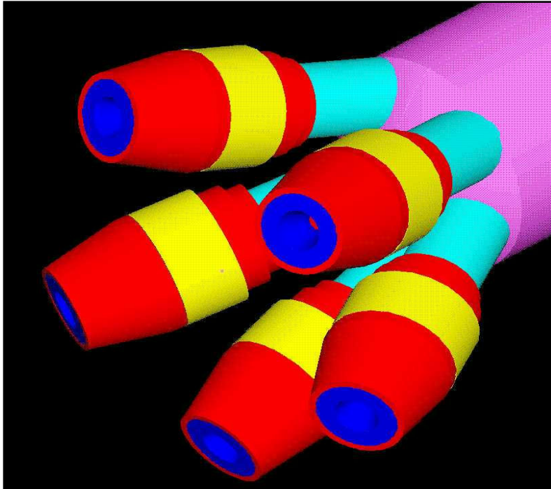
Isometric view of the nozzles, organ pipes, and central waterway of the bit
