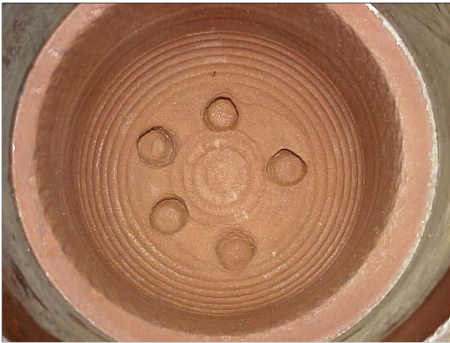
Erosion pattern created in Nugget Sandstone (18,000 psi UCS) during flow test
