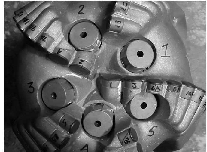
Bit near completion of testing indicating some erosion (Note installation of standard nozzles)
