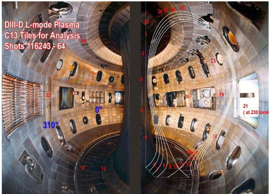
Divertor & SOL plasma characterized by Langmuir probes, Thompson scattering, spectroscopy, heat flux by IRTV.
