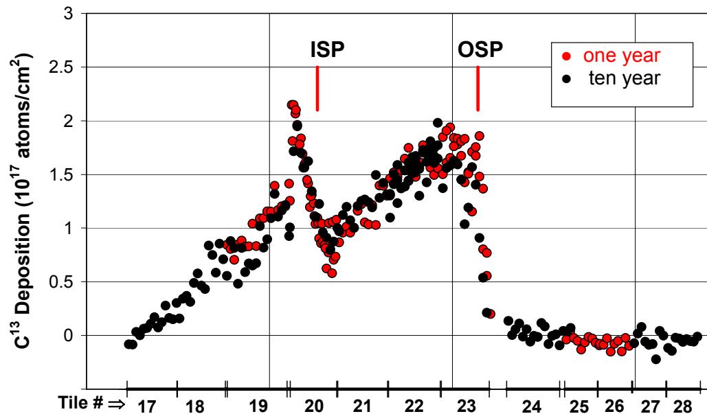
$^{13}\text{C}$  deposition was Toroidally symmetric
