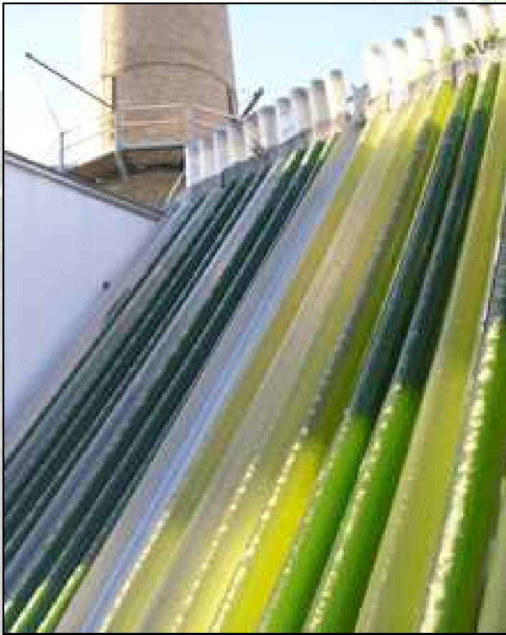
Algae bioreactor utilizing flue gas from MIT co-generation power plant.
