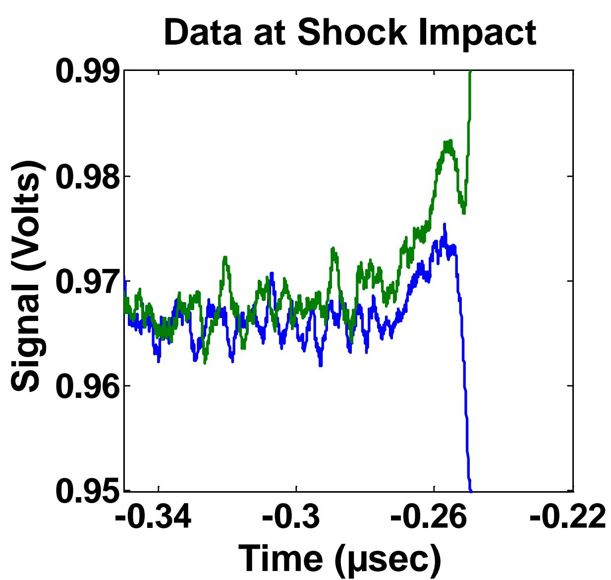
**Results:** Zooming in on initial impact, we see indication of a change in the gold dielectric. We can analyze the data at each point in time to give a plot of the gold’s dielectric as a function of time.
