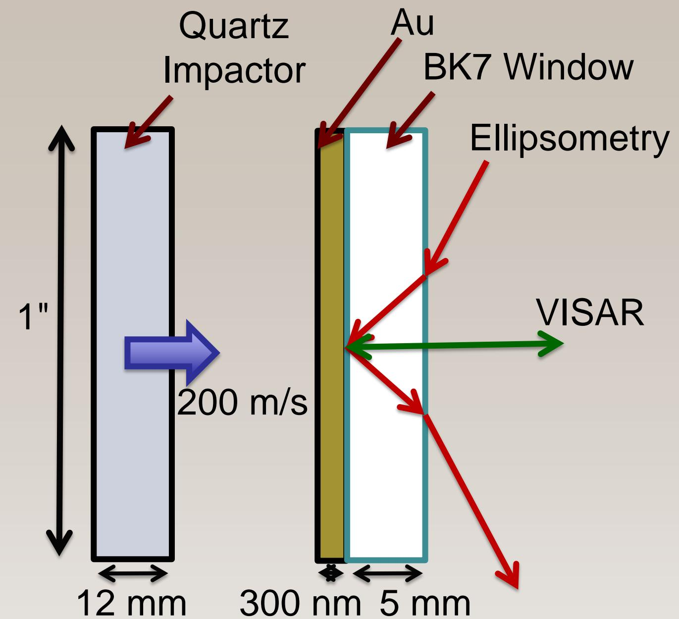
**Modeling Signals:** We model the anticipated results. In this case, a growing birefringent layer in the BK7 window due to the uniaxial compression causes a phase shift to steadily accumulate between the two independent polarization axis.
