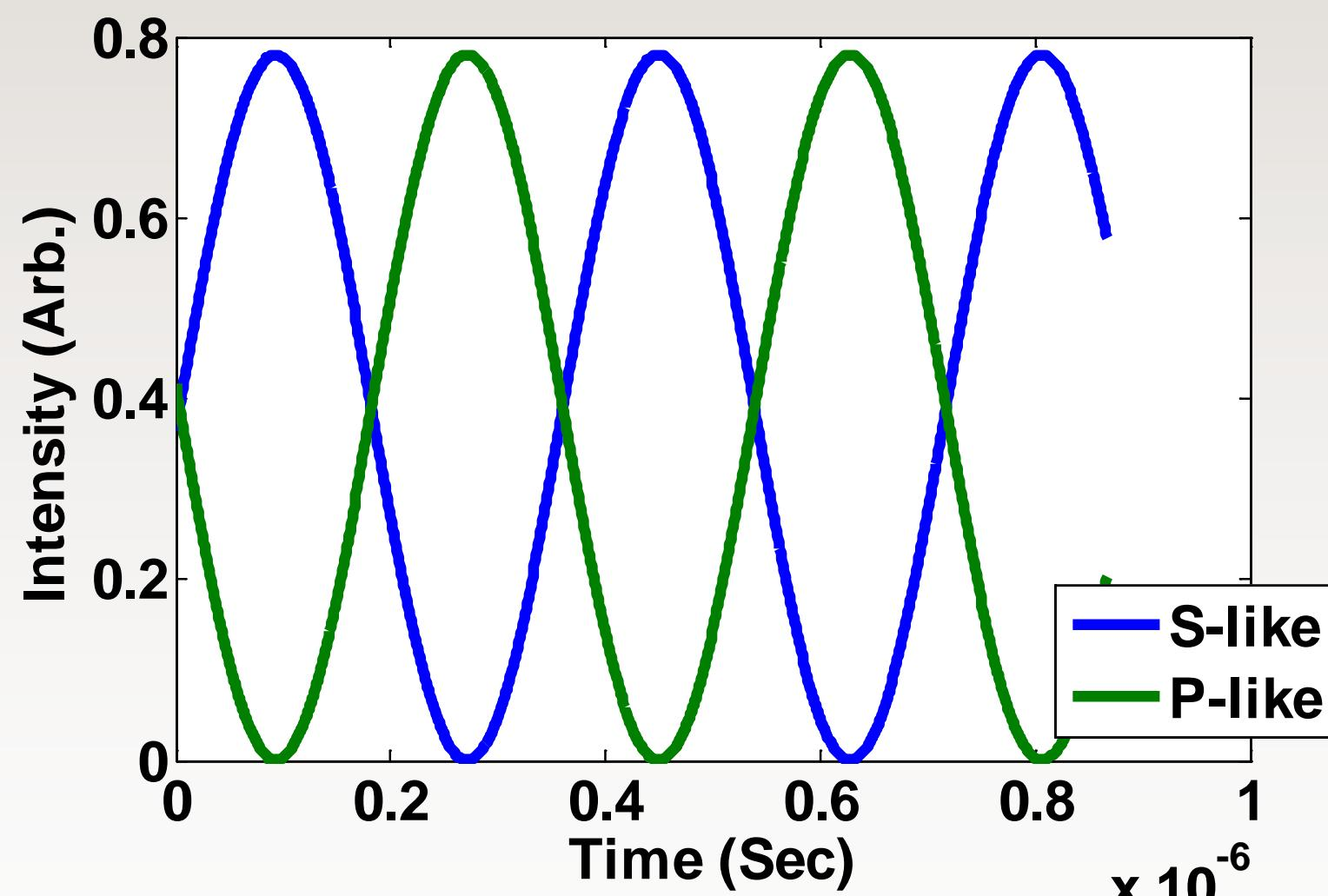
**Results:** Our experimental data resembles the modeled expected results, even showing a clear sign of the window birefringence being “erased” by the rarefaction wave after breakout (not included in model).
