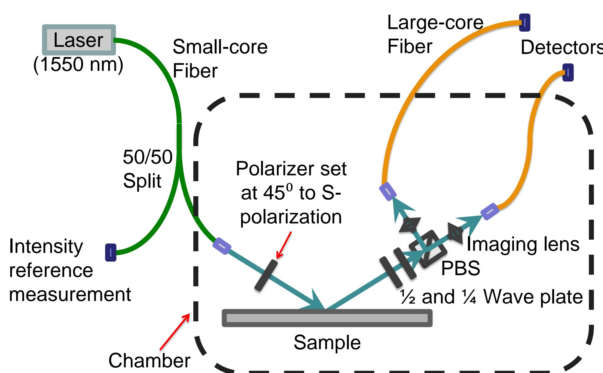
**Probe Design:** Open-beam optics set and analyze the polarization state while the fibers transport the light into and out of the chamber.
