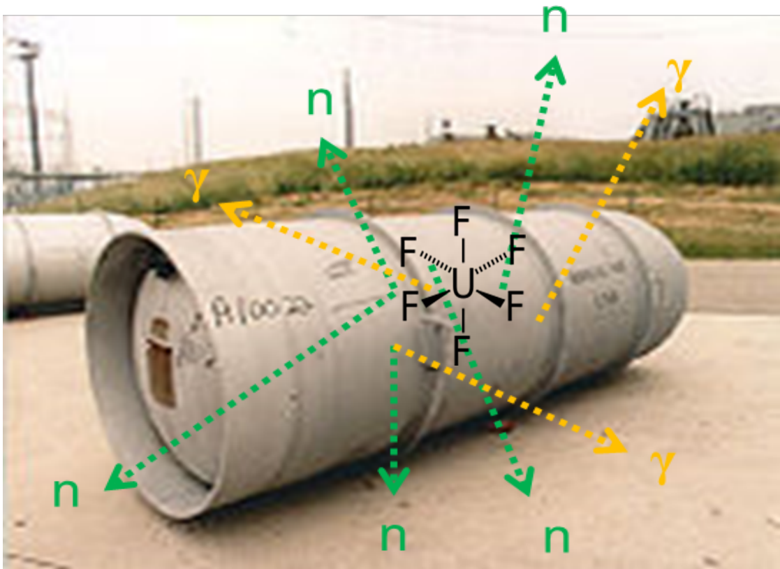
Fig. 1-2. Model 30B \text{UF}_6 container showing schematic neutron and gamma emission from the decays and reactions occurring within the container.
