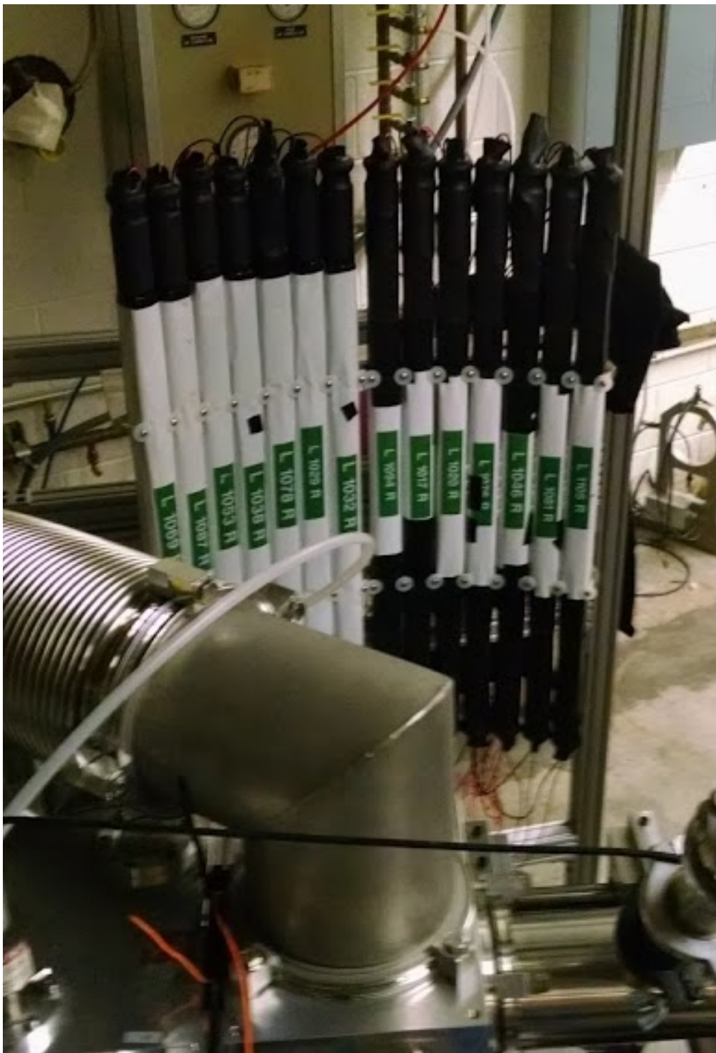
Fig. 2-14. VANDLE detector array setup (beam right, view from side) at ORNL for the fluorine-beam experiment.
