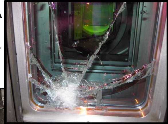
Damage to FOA debris shielding
