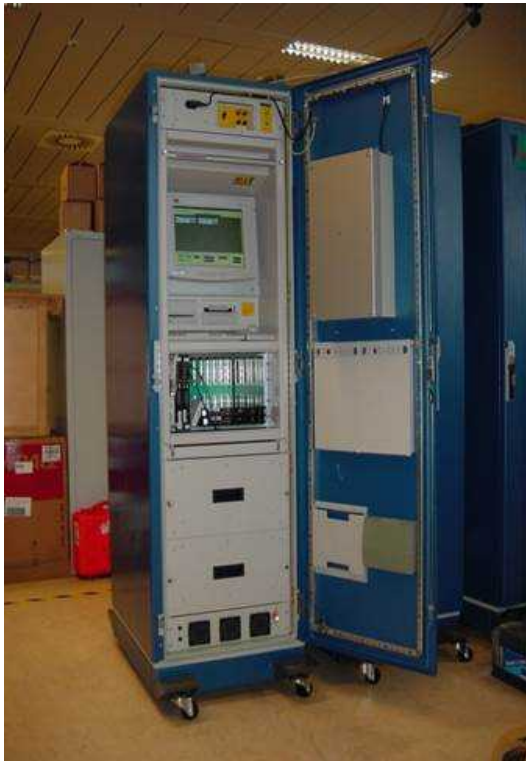
“Inspector owned” IAEA cabinet, painted using a powder process
