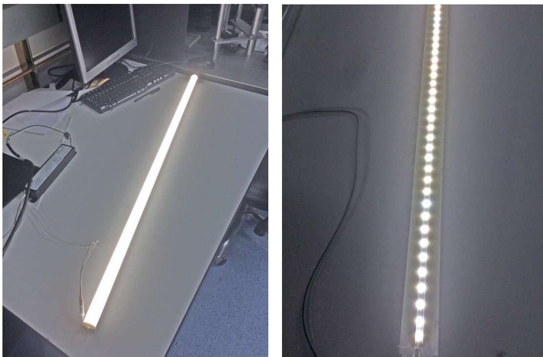
Fig 21. Photographs of the demonstration lamp with (left) and without (right) diffuser.
