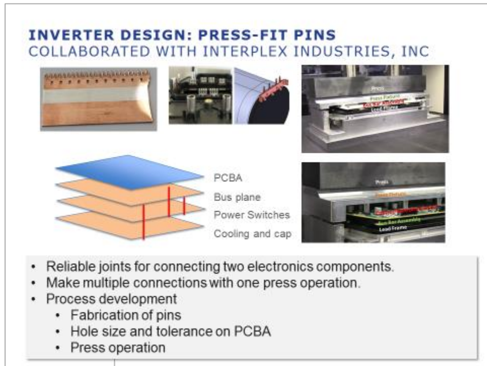
Figure 6 Press-Fit Pin Development
