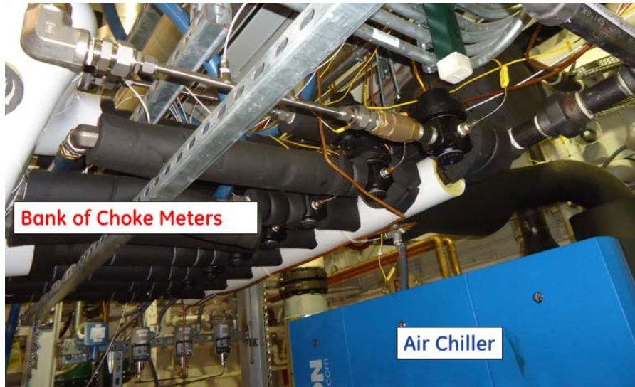
Figure 151: Bank of calibrated choke meters used to independently measure the flow rates of air and CO 2 , and the Air Chiller used for reducing secondary flow temperature
