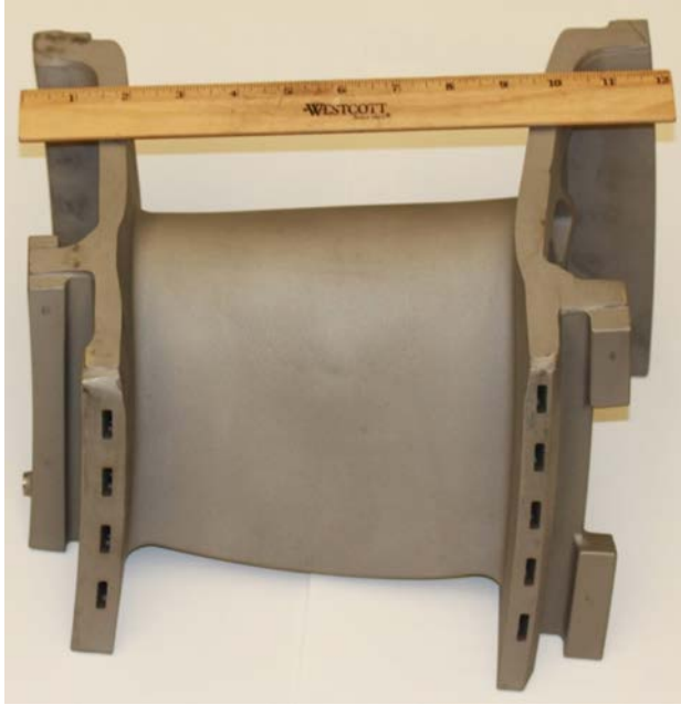
Figure 82: (a) A stage 1 nozzle cast with Rene' N2M.
