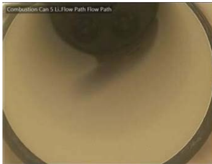
Figure 62: Improved TBC on a Combustion Liner after 3,644 hours in a Customer Unit
