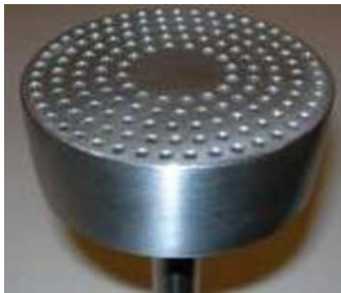
Figure 6: Early full-scale micromixer fuel nozzle used for single nozzle rig flame operability testing.
