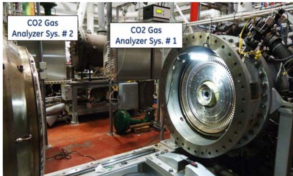
Figure 149: Exposed Rotor Blisk shows the rig's ability to exchange rim seal geometries on the rotor. The two CO2 Gas Analyzer systems used for CO2 sampling are shown in the background
