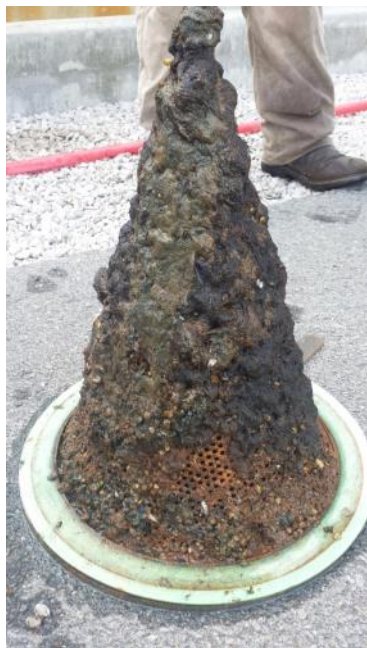
Figure 50. Fouled Water Pump Pre-screen.
