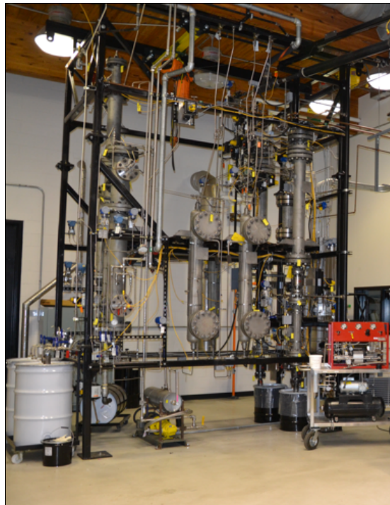
Gas conditioning platform. Filters are shown on far right, fixed bed reactors are in the center, and quench cooler and activate carbon filter are on the left.
