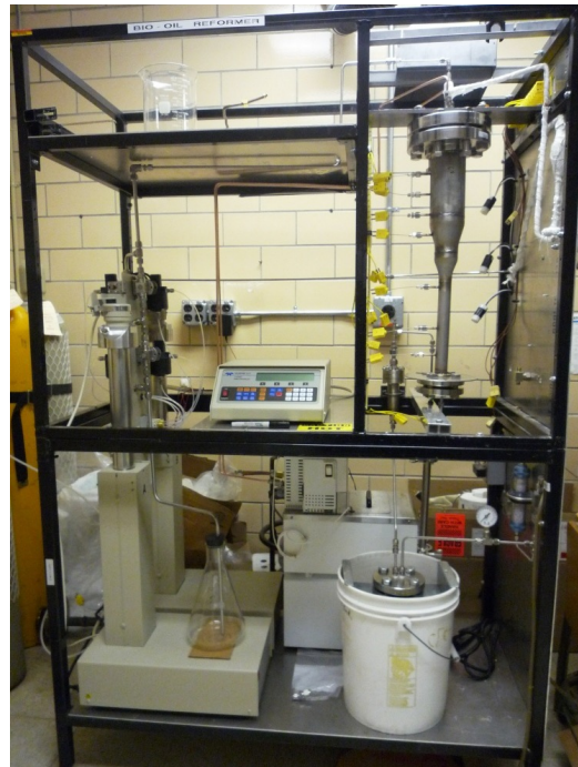
Figure 4. Assembly of the test rig to be used for bio-oil gasification study at atmospheric pressure.
