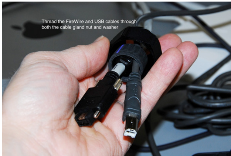
Figure 7. Firewire and USB cables are guided through washer and nut.
