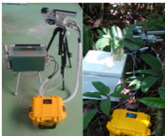
Figure 3. Portable photosynthesis and VOC emission system.
