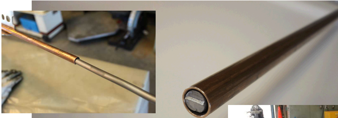
Initial Dimensions for Simulated Copper Fuel Rod Mock-up
