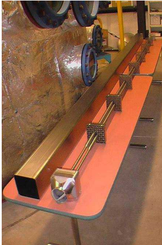
BWR channel, water tubes and spacers
