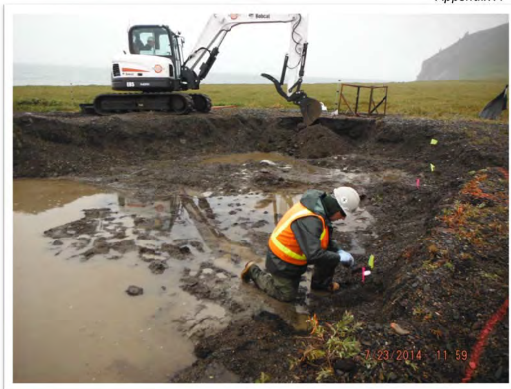
Photograph 27 – Sampler collecting excavation guidance sample 14PCC026SO and field duplicate 14PCC027SO. Laboratory results were below ADEC Method One cleanup levels and excavation activities were curtailed to the north. View to the west.
