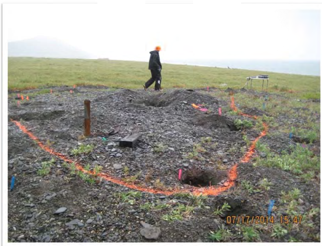
Photograph 21 – Surface soils at Test Hole Charlie were screened with a PID to estimate the area with POL-contamination (marked with spray paint). Casing is shown on left. View to the southeast.
