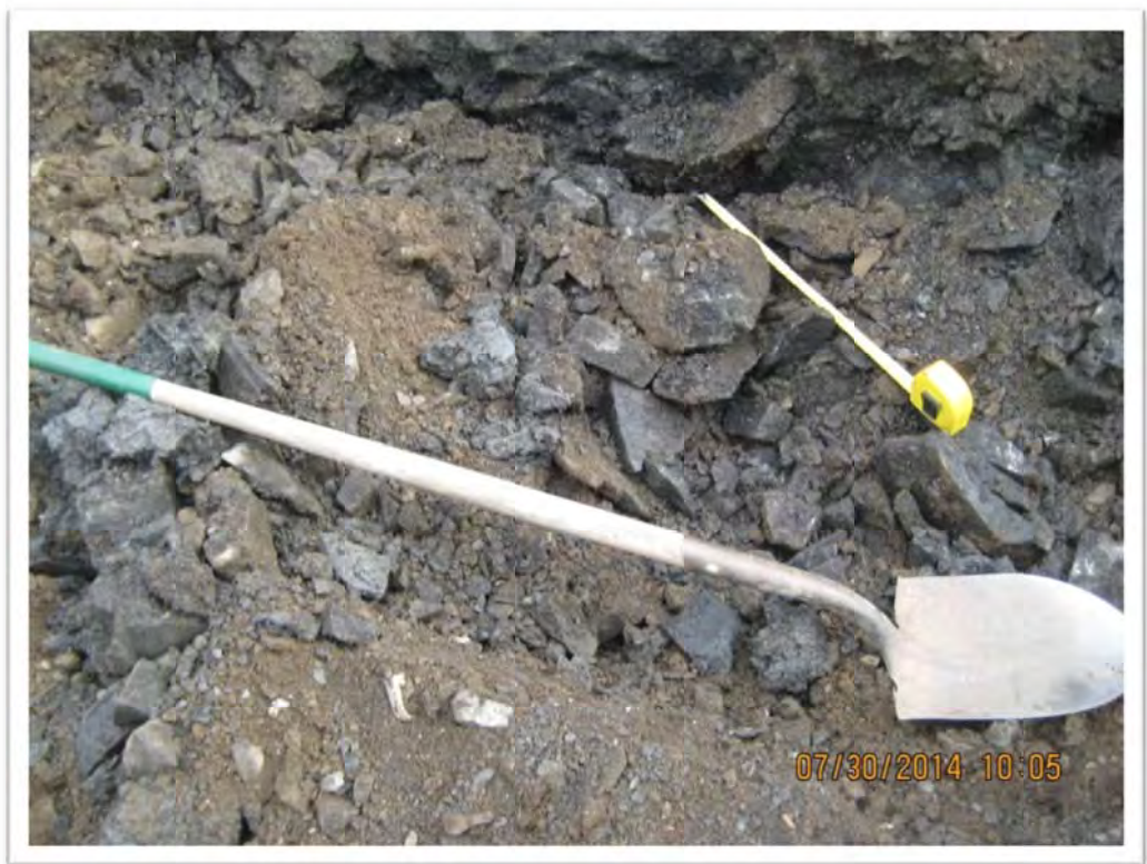
Photograph 46 – Rock size increased with depth of excavation; rocks up to 10 inches in diameter were encountered. Permafrost was encountered at approximately 5 feet below ground surface and limited vertical excavation.
