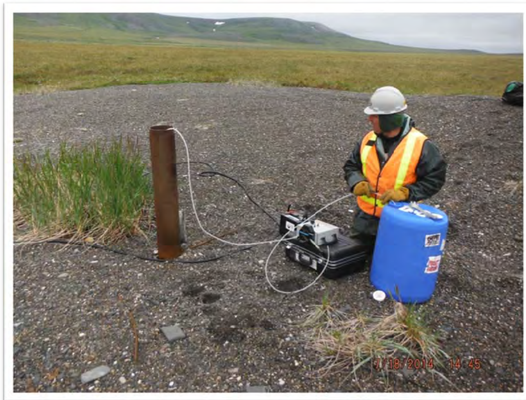
Photograph 7 – Approximately 4.5 gallons of water were pumped from the Test Hole Able casing. View to the northwest.
