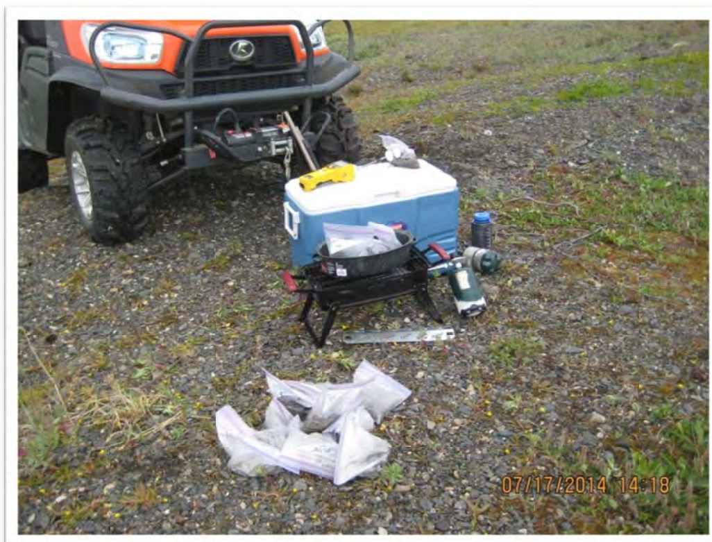
Photograph 25 – Screening samples in sealable plastic bags were heated in a water bath prior to measuring headspace with a PID. Excavations were guided using PID screening results.
