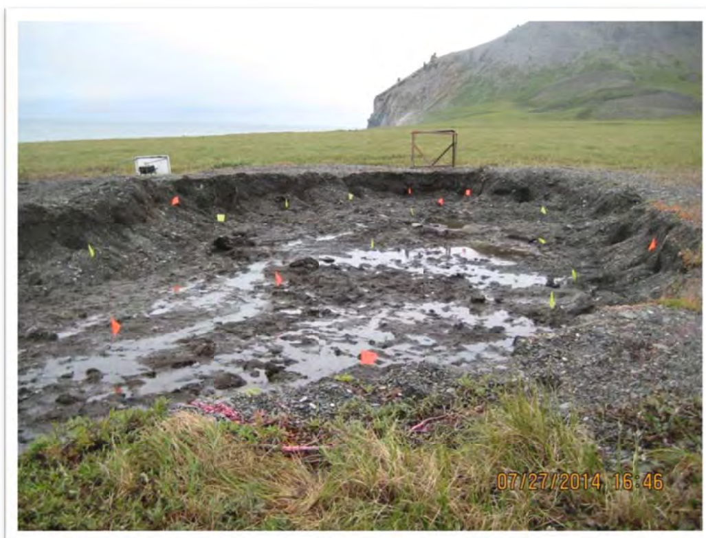
Photograph 29 – Northern half of Test Hole Charlie excavation. Yellow flags represent PID screening locations. Orange flags represent PID screening and laboratory sample locations. View to the west.
