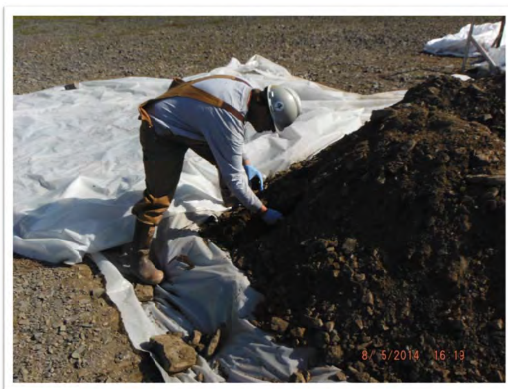
Photograph 50 – Sampler collecting soil samples from a stockpile. Five locations from each stockpile were field screened, and laboratory samples were collected from the location with the highest PID result.
