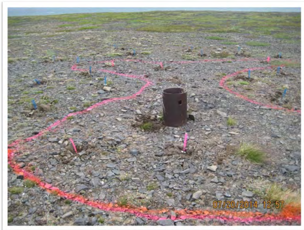
Photograph 43 – POL-contamination in surface soil at Test Hole X-1 was marked with spray paint. The actual excavation extended further than the surface contamination. The site is located on a sparsely vegetated hilltop. View to south.
