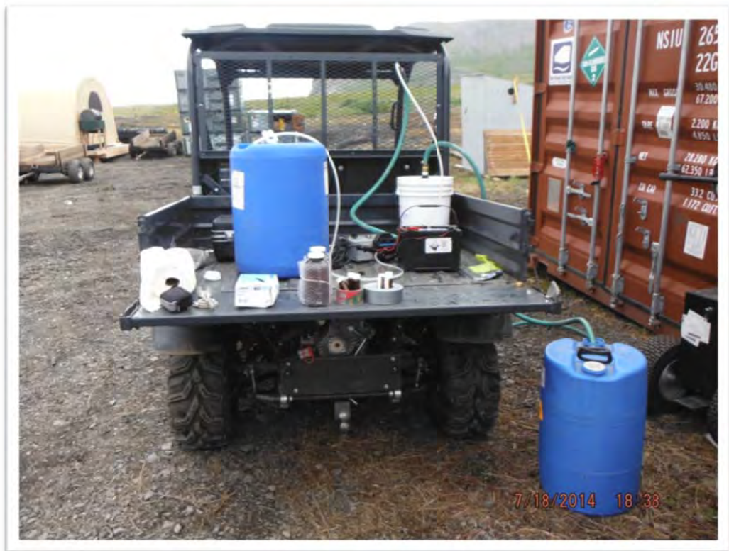
Photograph 8 – Approximately 9 gallons of casing water was treated collectively with granular activated carbon prior to surface discharge. Representative samples were collected pre- and post-treatment. View to the west.
