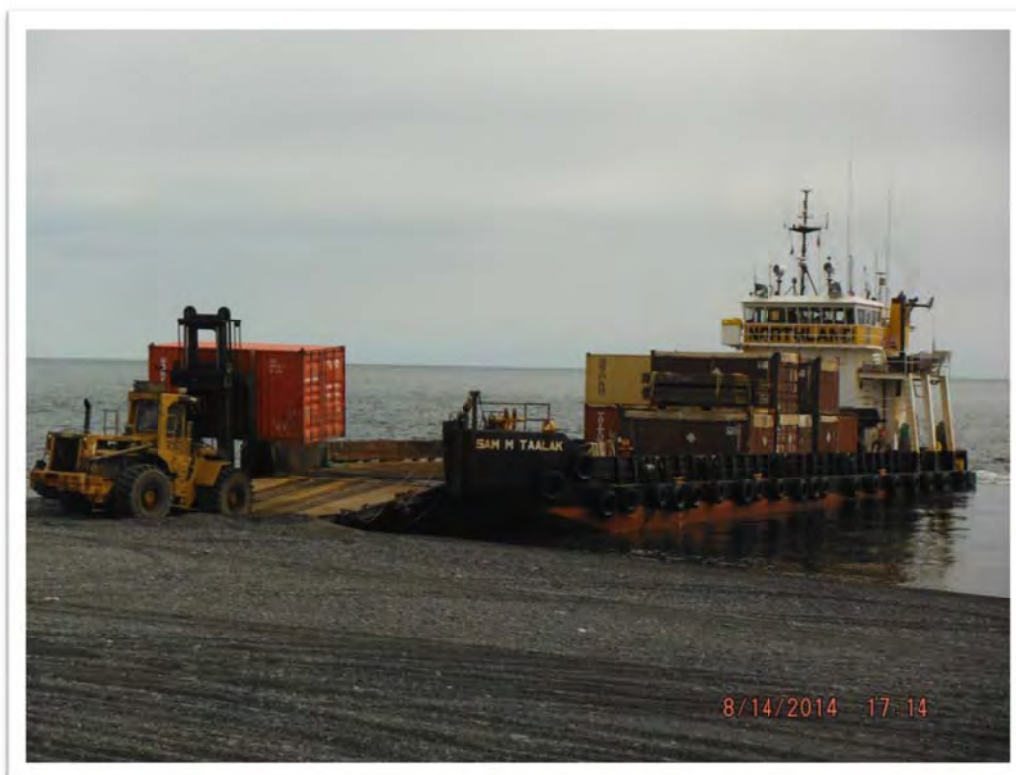
Photograph 58 – Loading connex boxes onto 140-foot landing craft. A total of 41 connexes filled with POL-contaminated soil were removed from the site. View to southeast.
