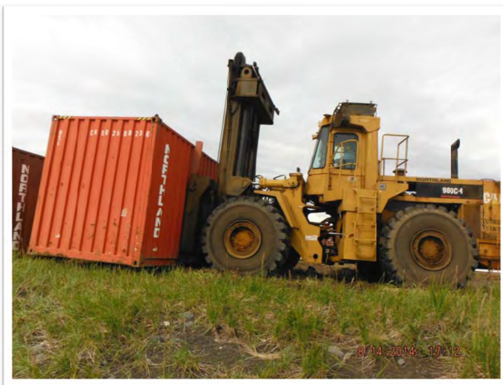
Photograph 57 – A 980C-4 Caterpillar equipped with forks was used to move this container from the West Staging Area onto the landing craft. View to north.
