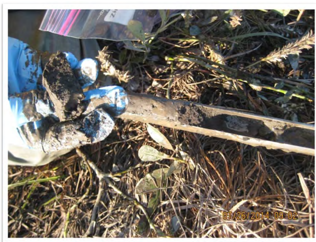
Photograph 28 – Due to frozen soils and standing water, several floor samples on the southern side of Test Hole Charlie were collected with a hand-driven probe as shown in this photograph. View to southeast.
