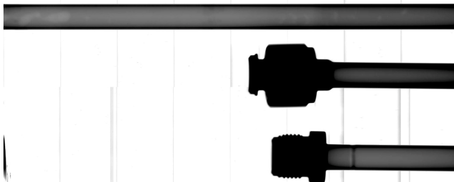
Figure C- 13: X-ray CT image at valve end (reference angle: 0°) of the three sample tubes in “saturation” mode at 213 kVp, 2.5 mA, It=4.0 sec (top: sodium filled tube, middle: air tube, and bottom: water tube).
