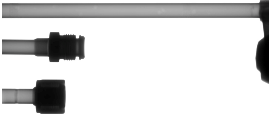
Figure C- 5: X-ray CT image at plug end (reference angle: 0°) of the three sample tubes in “saturation” mode at 170 kVp, 3.5 mA, It=4.0 sec (top: sodium filled tube, middle: air tube, and bottom: water tube).
