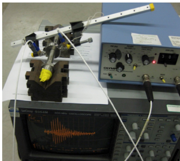
Figure 4-2: High-frequency ultrasonic system and experimental setup
