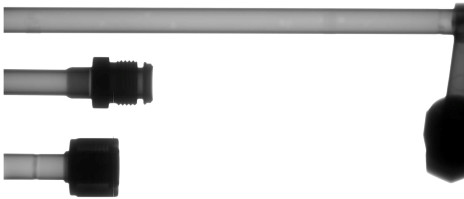
Figure C- 6: X-ray CT image at plug end (reference angle: 90°) of the three sample tubes in “saturation” mode at 170 kVp, 3.5 mA, It=4.0 sec (top: sodium filled tube, middle: air tube, and bottom: water tube).
