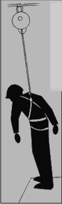
Worker using a self-retracting lifeline (left and right).
