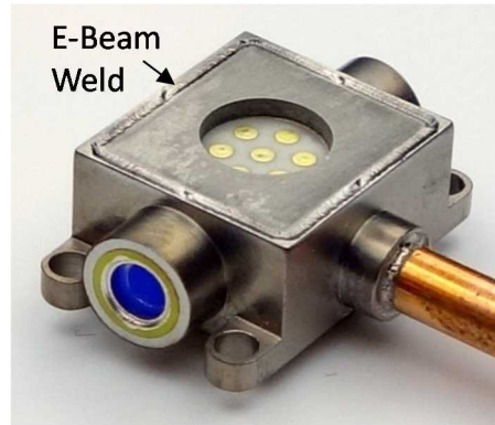
Figure 4. Photograph of the completed hybrid metal-ceramic vacuum package. Note the e-beam weld seam.
