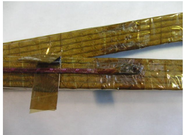
Figure 5.18: Detail of thermocouple attached to stator coil
