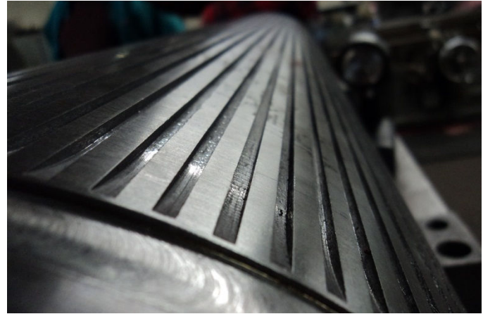
Figure 5.23: Detail of fins machined on housing OD
