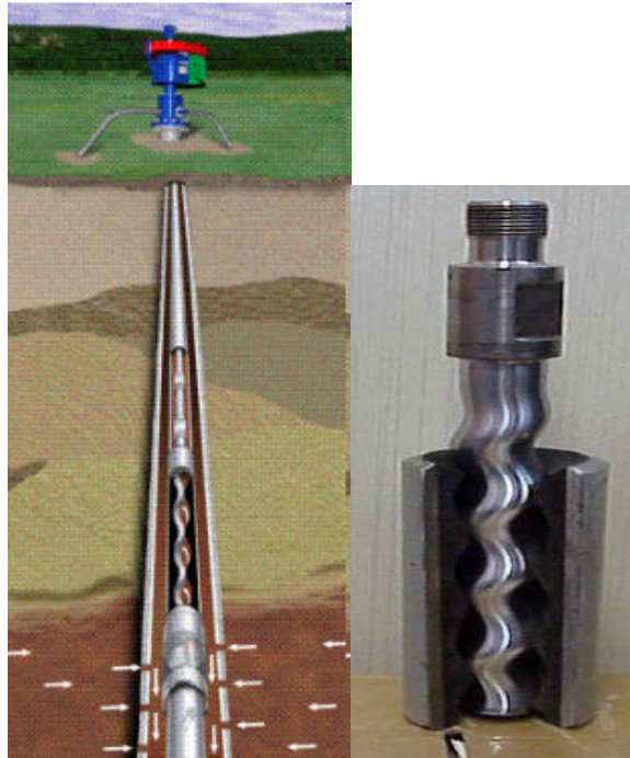
Figure 2.8 - Progressing cavity pump configuration; close up of rotor / stator. (courtesy: World Oil, July 2006)
