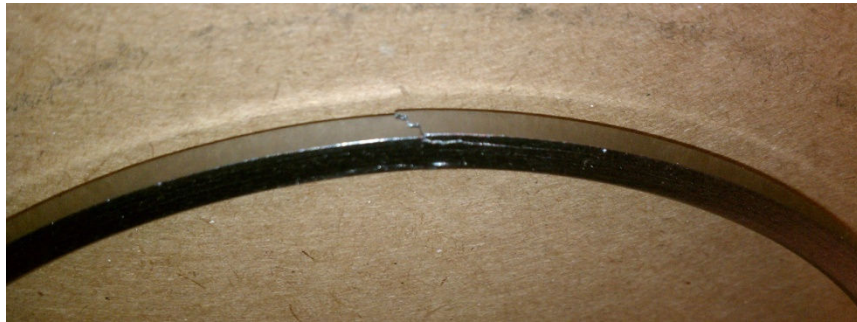
Figure 5.38 – Overall seal test data and damaged secondary seal
