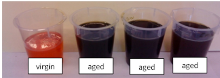
Figure 5.41 - Aging studies in oils. The color of the oil becomes dark when it is heated to 350°C at 300 bar.
