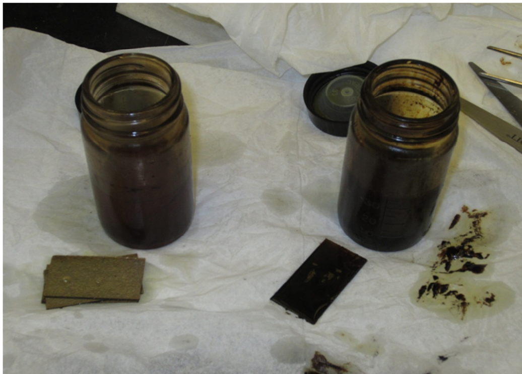
Figure 5.43 - Oil comparison after thermal aging at 330°C and 400 psi for three weeks; oils (A) and (B) in the left and right containers respectively. The insulation materials tested show different surface characteristics due to deposited black-substance. The insulation on the left has a clear surface.
