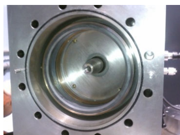
Figure 5.36 – Seal before and after assembly in 5-inch rig
