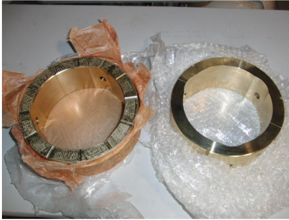
Figure 5.15: (Left) Radial-thrust bearing showing thrust faces; (Right) radial bearing
