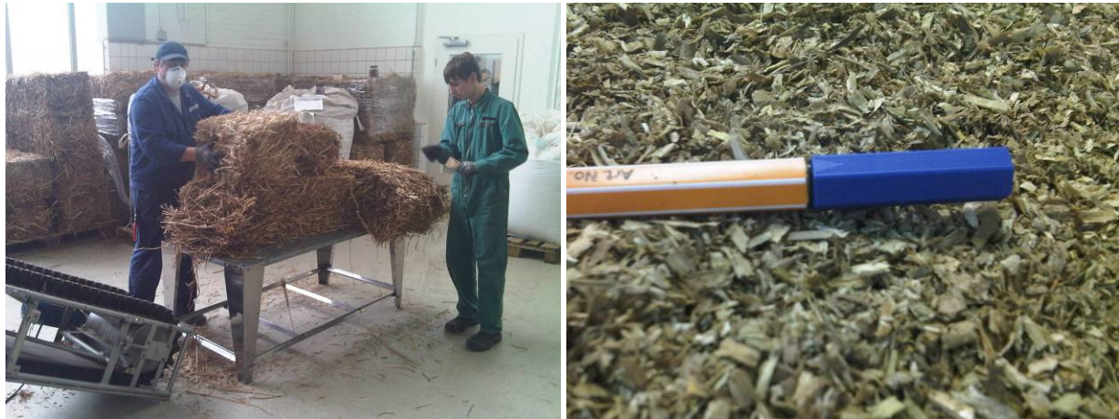
Figure 3. Switchgrass bales being loaded onto a conveyor belt and milled switchgrass after grinding
