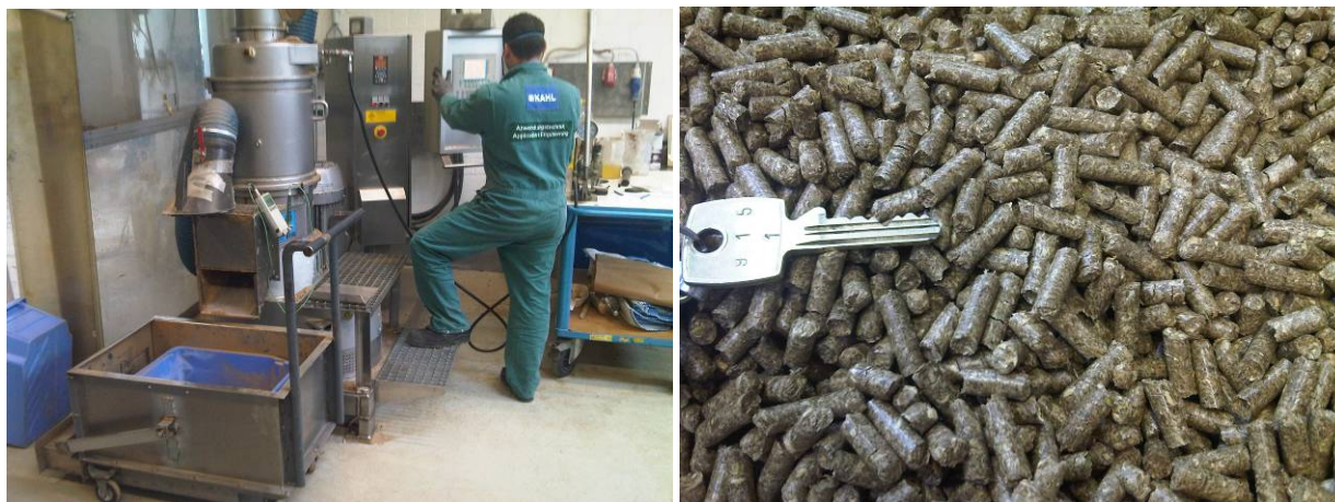
Figure 4. Pellet mill test stand at Amandus Kahl and pelletized switchgrass using a 6mm die
