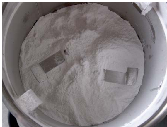
Crushed feed, plenty of surface area, ready for dissolution
