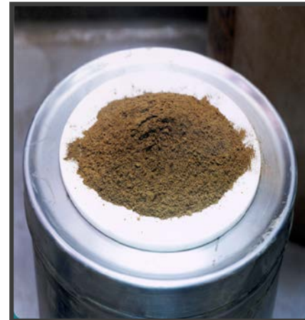
Pu/Am Oxide, high Pu/Am purity, highly stable/storable
