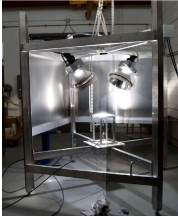
Fig. 3. Solar simulator with two lamps (3.6 kW) during a flux-mapping characterization
