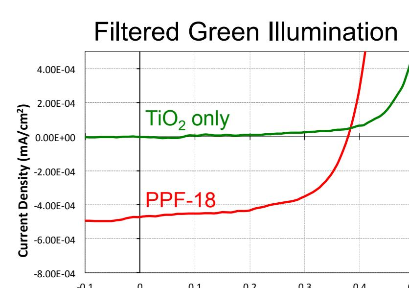
Initial test cells show measureable photocurrent from MOF-based DSSCs! Green light illumination confirms the source of the photocurrent is from the porphyrin used to make the MOF.
