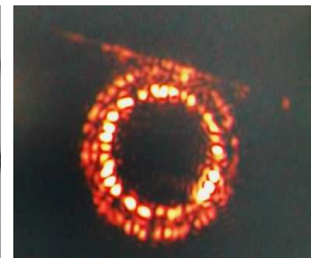
SHG observed on visible camera when pumping with infrared light
