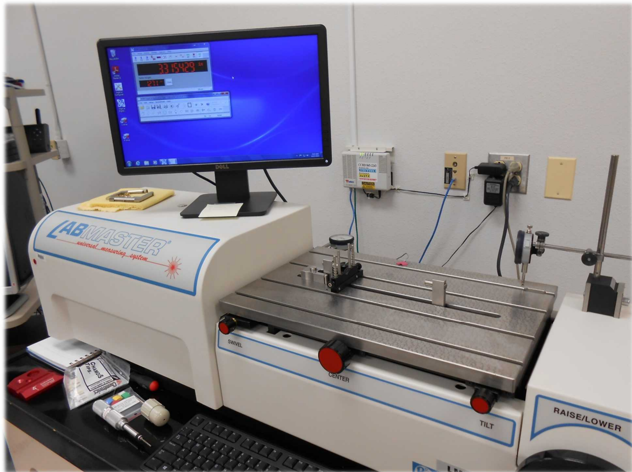
Figure 4: Photograph of the Horizontal Measurement System. The standard diameter parallel anvils are shown. Note that two dial indicators were added by the authors to provide immediate feedback when changing table position.
