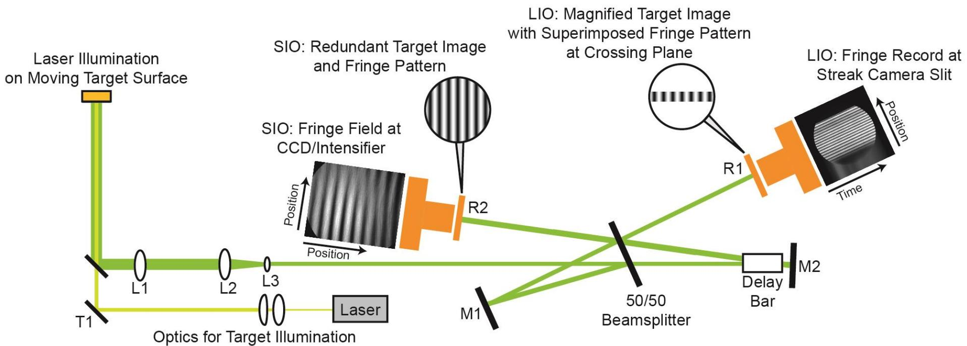
Varied settings: Camera recording time, Velocity-per-fringe, Image magnification and fringe density
