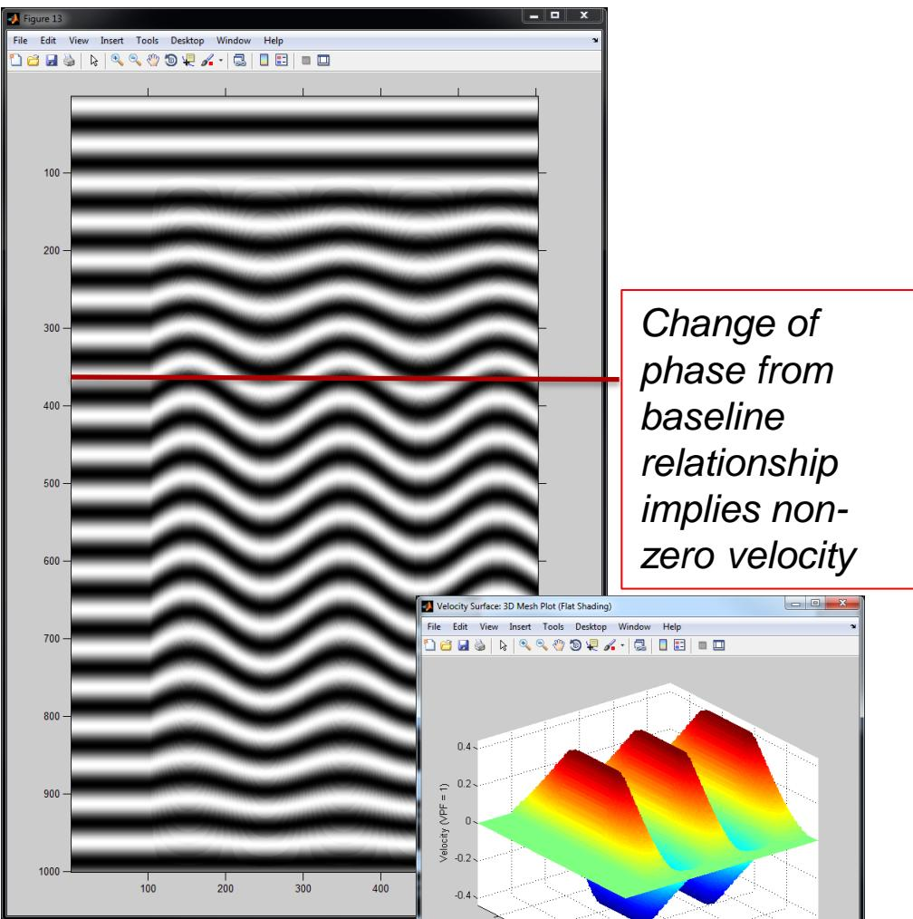
4. Calculate velocity surface in space and time
