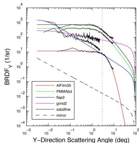
Diffuse and Patterned Surfaces with Associated Bidirectional Reflectance Distribution Function (BRDF)
