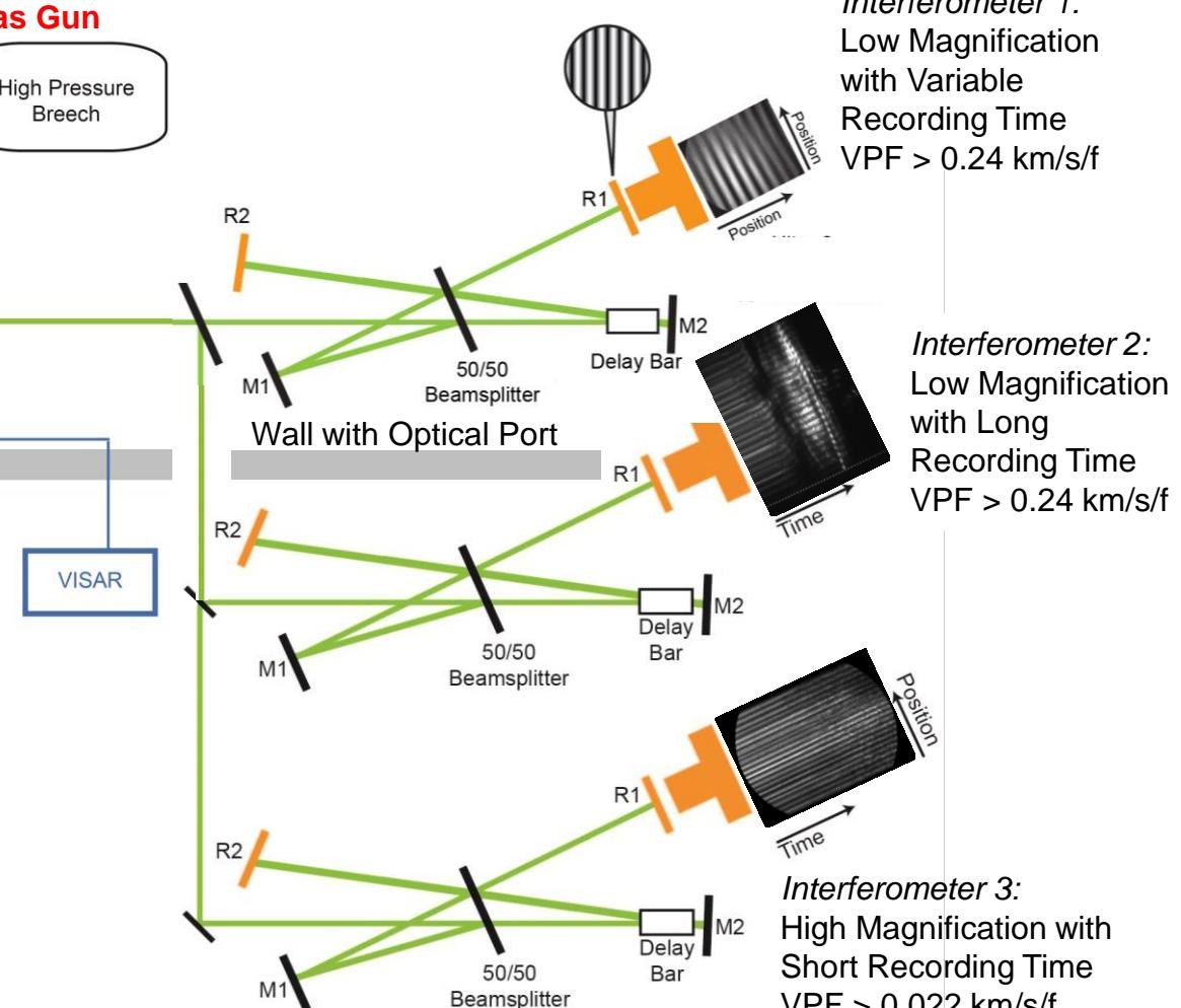
Example: Line- and Surface-imaging ORVIS on planar impacts of fused silica
