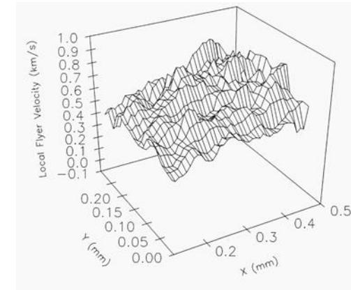
Stop motion of fringe field from laser-driven flyer launch
