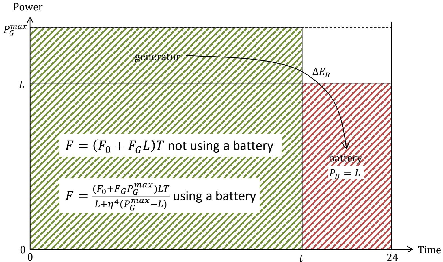
A battery saves fuel with a small load  $L < \tilde{L} = \frac{F_0}{F_G} \frac{\eta^4}{1 - \eta^4} \cong 3 \frac{F_0}{F_G}$
