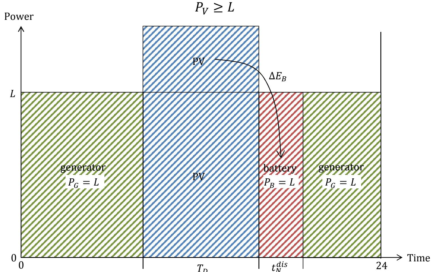
$$F = (F_0 + F_G L) \cdot \left[ T_N - \min \left( T_N, \frac{\eta^2 E_B}{L}, \frac{\eta^4}{L} (P_V - L) T_D \right) \right]$$
