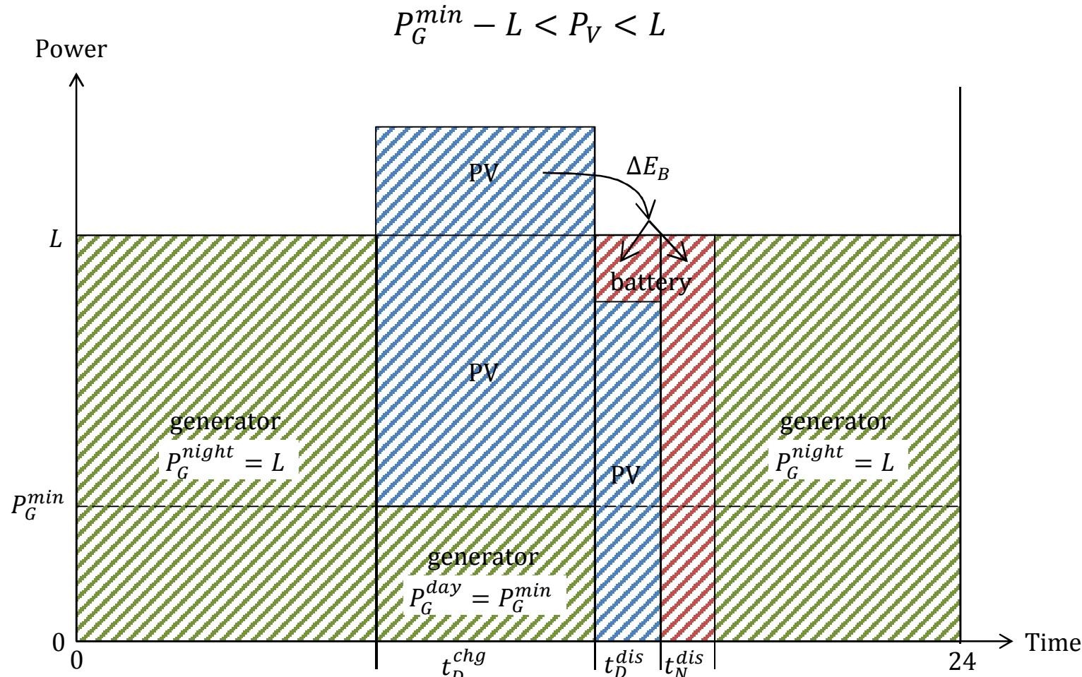
$$F = (F_0 + F_G L)T_N + (F_0 + F_G P_G^{min}) \frac{T_D(L - P_V)}{(L - P_V) + \eta^4(P_G^{min} + P_V - L)}$$
