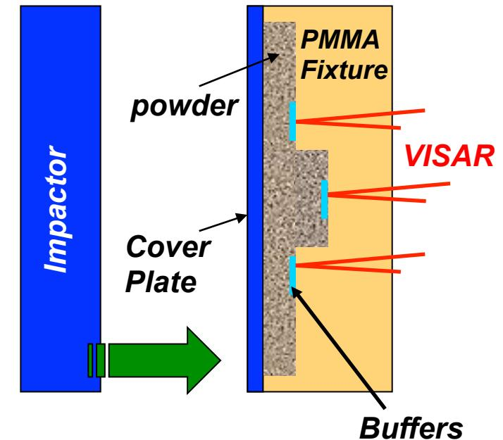
stepped sample for accurate shock velocity and uniform powder density; sealed capsule allows fluid / powder mixtures
