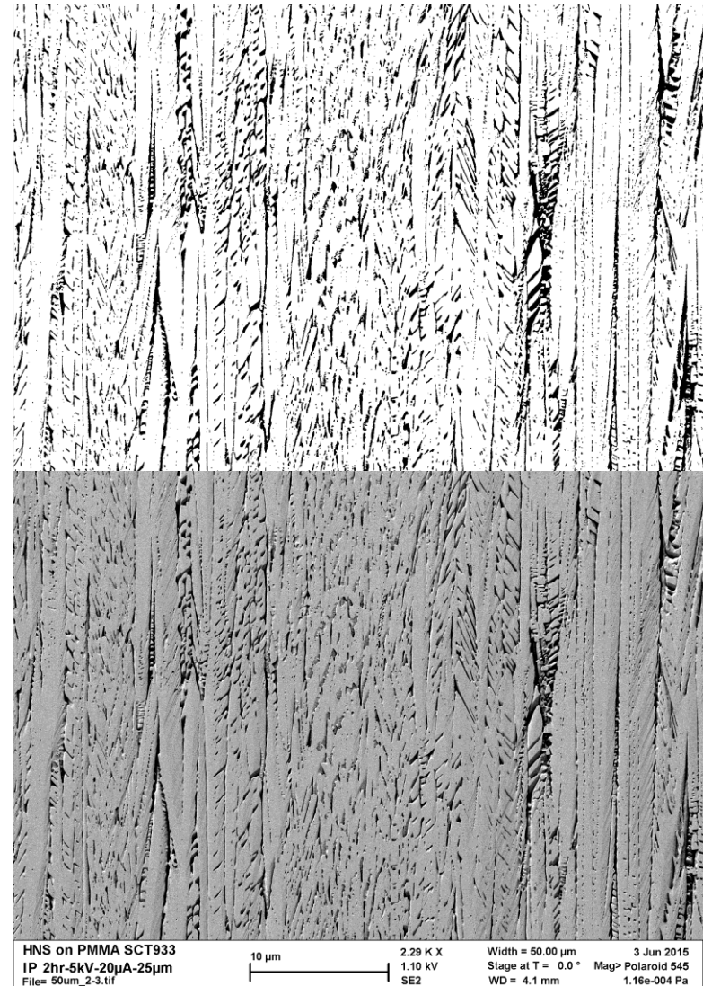
Raw and binarized SEM images of HNS films deposited at 10 °C (left) and 45 °C (right)
