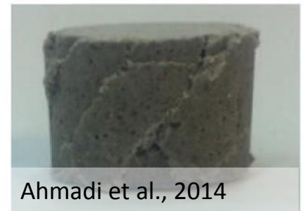
Figure 7. Shear cracks formed during plateau region on syntactic foam.
