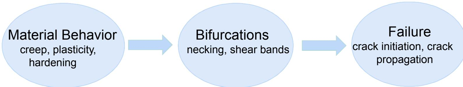
Accurate predictions of ductile tearing in metals
