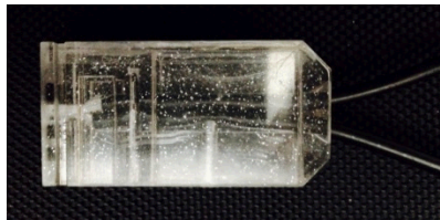
Figure 1: Cobra 5 Seal with Embedded Hematite. Photo courtesy Sandia National Laboratories.
